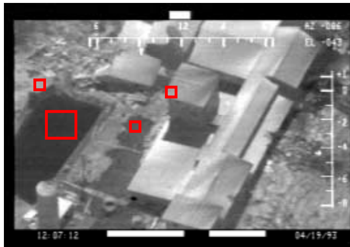
Figure 5.35. Selected regions for normalization of grey levels illustrated in one of the frames, on the platform near the swimming pool, on the central tower roof, on the lawn in the courtyard and on the water surface in the swimming pool. An additional area was tracked on the soil of the red side.
