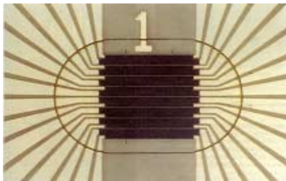
Figure 5.2. A SPRITE/TED array, from [Baker] p. 153.
