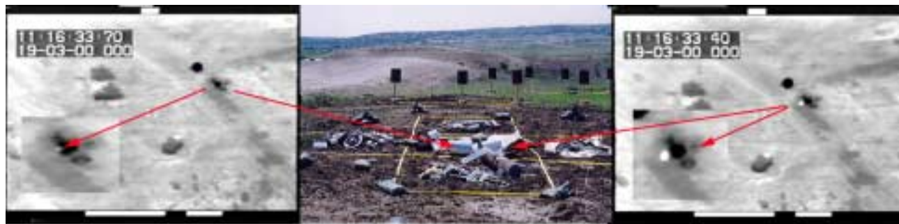
Figure 5.28. Debris causing reflections during the Fort Hood flight trial on the Lynx FLIR imagery. A flash that was small, elongated and short in duration (left) and a flash that was larger and longer in duration (right).
