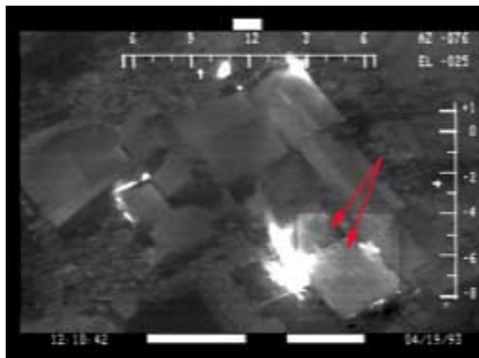
Figure 5.25. Several hot spots on the cafeteria roof, 12:10:43 (highlighted square and at red arrows and other locations on the roof).
