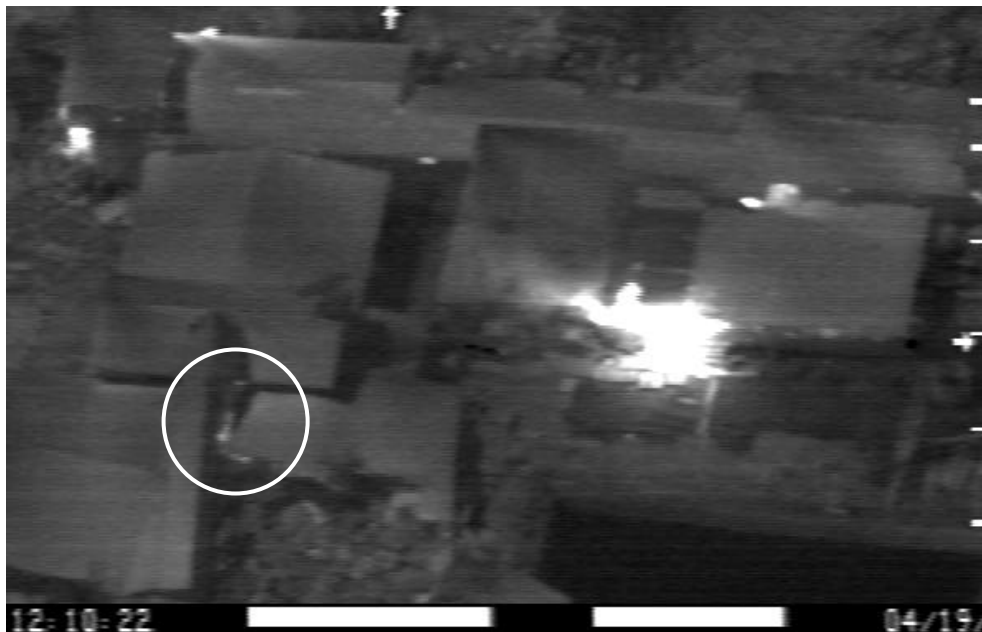
Figure 2.7 FLIR image from 12:10:22. A strong heat image started to appear at the eaves of the collapsed catwalk at 12:10:21. It developed quickly into intense flaming.
