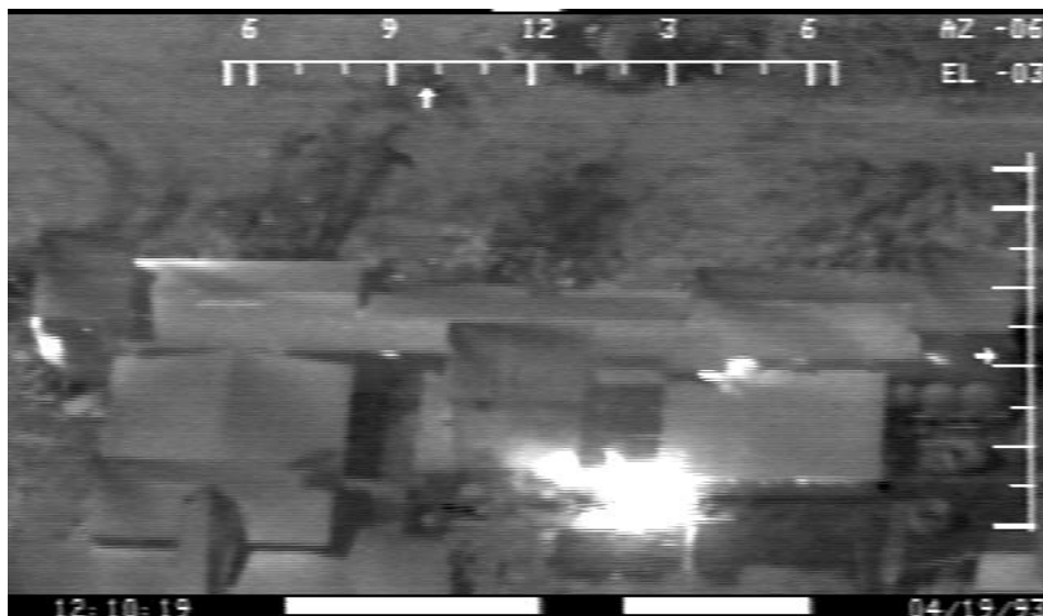
Figure 3.1 FLIR image 12:10:19. Hot gases are indicated in several places of the second floor and along the Black Side of the cafeteria.
