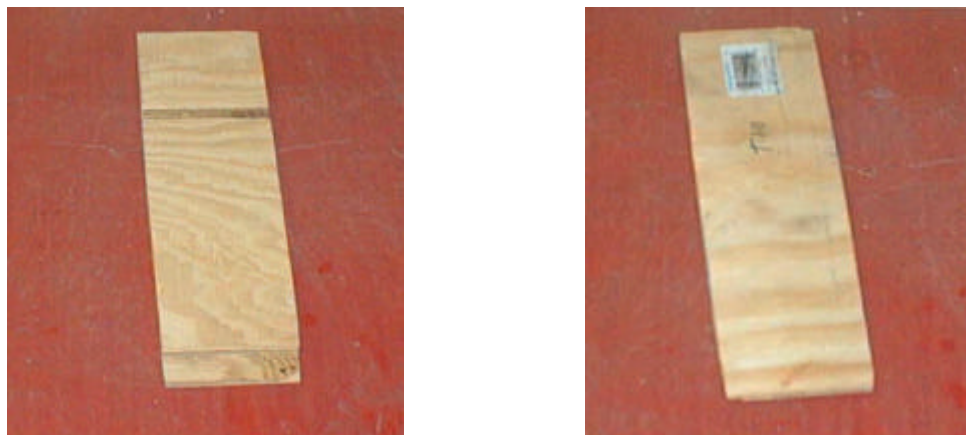
Figure 1 The received sample of plywood 5/8” with external side grooves. The left photo shows the external side. The un-grooved side was exposed to the radiant heat.
