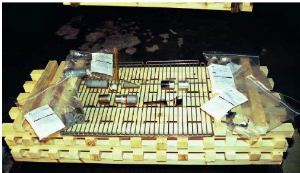
Figure 2 The specimens were placed inside the wood crib. Item 1 lower/right, item 2 upper/right, item 3 upper/left and item 4 lower/left. (The bags at the sides contain the duplicates of the test samples. The duplicates were removed prior to completion of the wood crib.)
