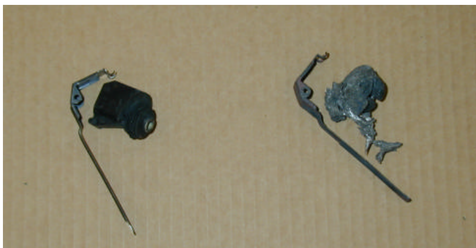
Figure 5 Item 1, Evidence Label No. A00811749 - Lever and cap from expended hand delivered flash bang grenade, not tested and tested, respectively.
