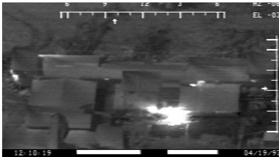
Figure 4.1 FLIR image 12:10:19. Hot gases or flames are indicated in the windows of the staircase and of the adjacent room.
