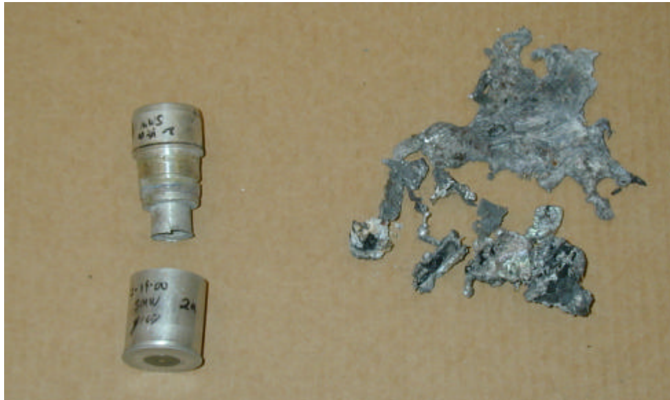
Figure 6 Item 2 Evidence Label No. A00811748 - Forty millimeter flash Bang casing and projectile fired from a M-79 Grenade Launcher, not tested and tested, respectively.
