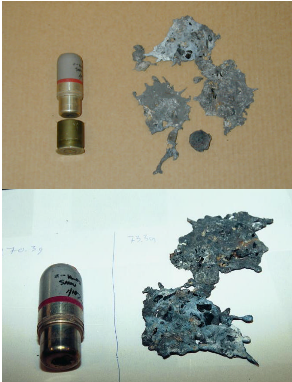
Figure 8 Item 4 Evidence Label No. A00811102 - Forty millimeter XM651E1 casing (military rounds) and spent projectile, not tested and tested, respectively. The lower picture shows the projectile only.
