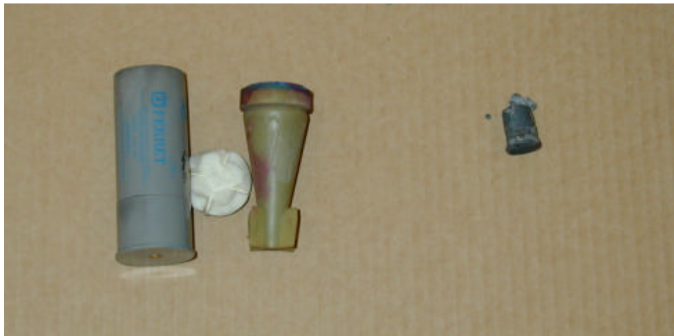
Figure 7 Item 3 Evidence Label No. A00811108 - Forty millimeter Ferret casing, wadding and projectile, not tested and tested, respectively. The remainder is a piece from the casing.
