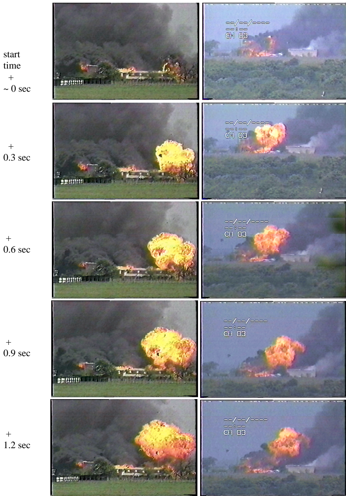
Figure 7.1. Illustration of BLEVE Development from Two Camera Positions
